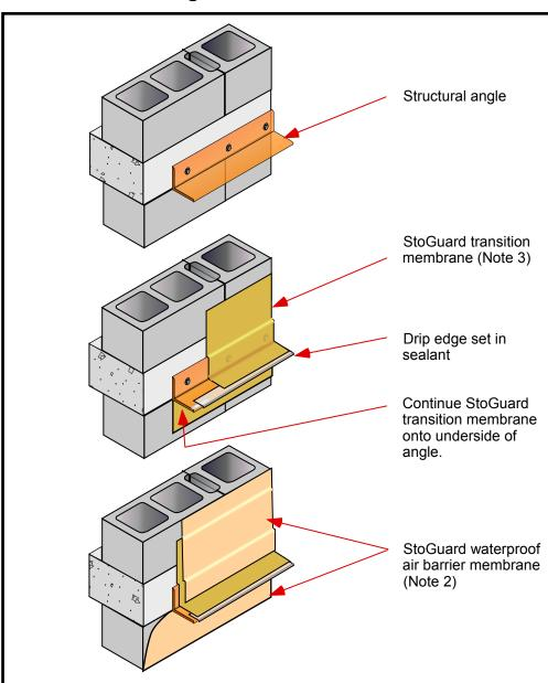
waterproof air barrier membrane and transition materials. When a skim coat of the leveling material is to be applied only one coat of the waterproof air barrier membrane is typically required (refer to Sto Detail 21.00b). Use a site mock-up and site tests as the basis for the work. Property of Sto Corp. All Rights Reserved
